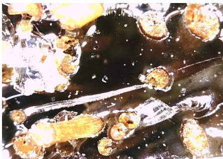
Gambar 7. Foto makro serat searah curing 30 menit
