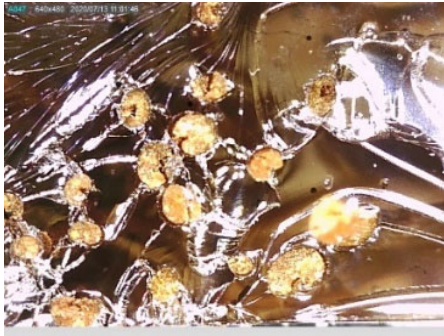
Gambar 5. Foto makro serat searah curing 50 menit
