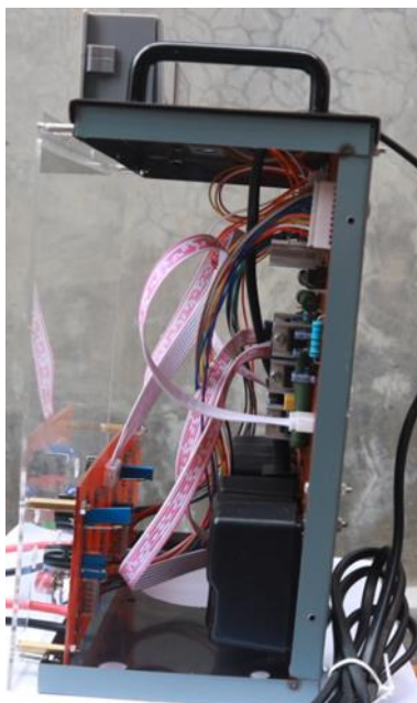
Gambar 2. Purwarupa rangkaian Wheatstone Bridge, Power supply, dan Amplifier
