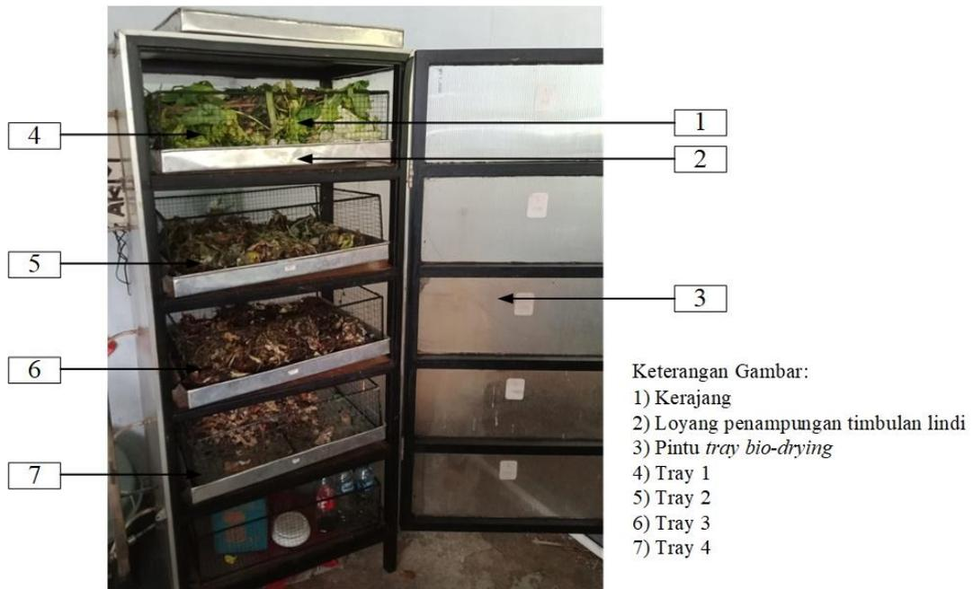
Gambar 1. Reaktor Tray Bio-drying
