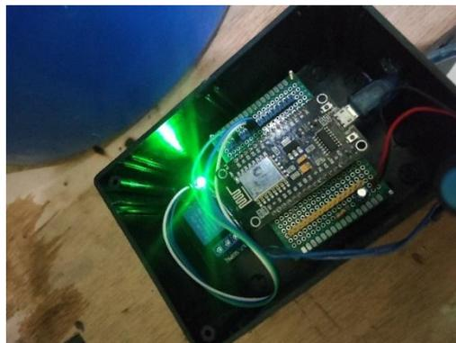
Gambar 10: Kondisi Relay Ketika HIGH Pompa Air DC OFF
