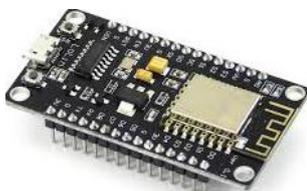
Gambar 5: NodeMCU lolin V3 [5]
