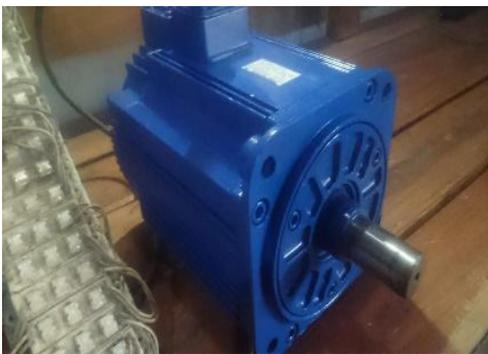
Gambar 1: Generator Magnet Permanent [2]
