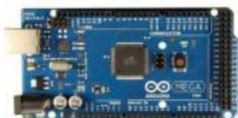
Gambar 5 : Arduino Mega 2560 [5]
