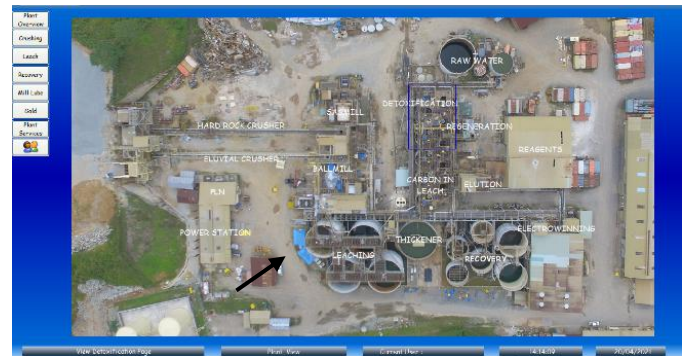
Gambar 2: Plant View di citect SCADA sebelum penambahan halaman baru
