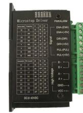
Gambar 2: Driver Motor Stepper
