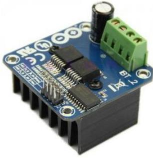
Gambar 6: Modul Driver BTS7970A
