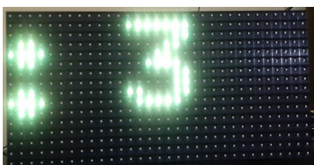
Gambar 8 Tampilan Lanjutan Display P10 LED RGB Dot Matrix
