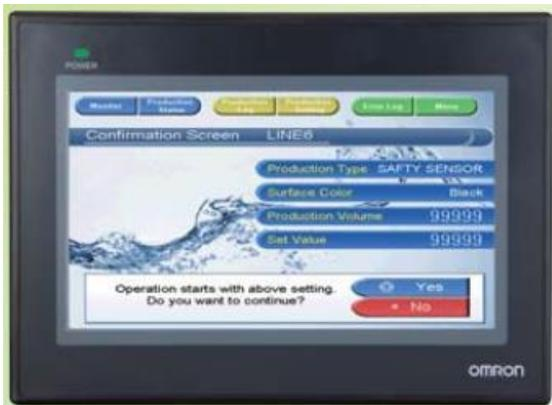
Gambar 3: HMI Omron NB7W-TW000B [10]
