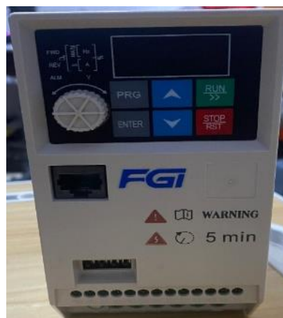
Gambar 3: Variable Speed Drive
