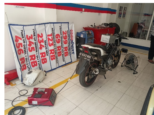
Gambar 2. Setting Peralatan Pengujian Emisi Gas Buang
