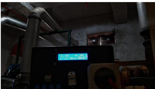
Figure 16. Temperature Conditions on Hardware Box and Cooling Fan Auto Turn On
