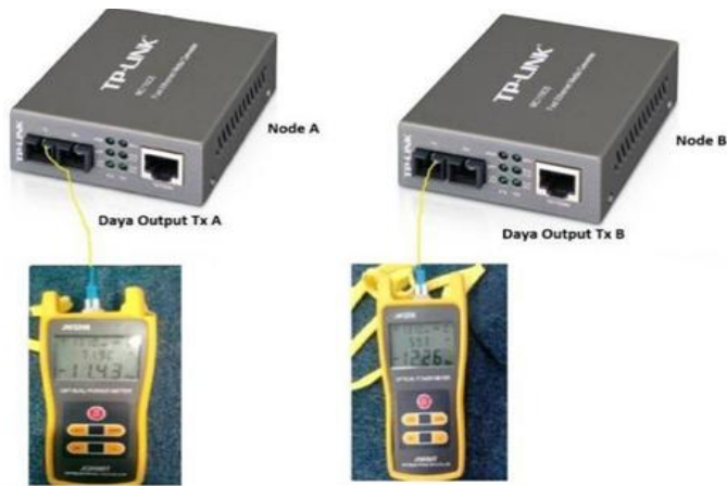
Figure 10. Media Converter Output Power Measurement
