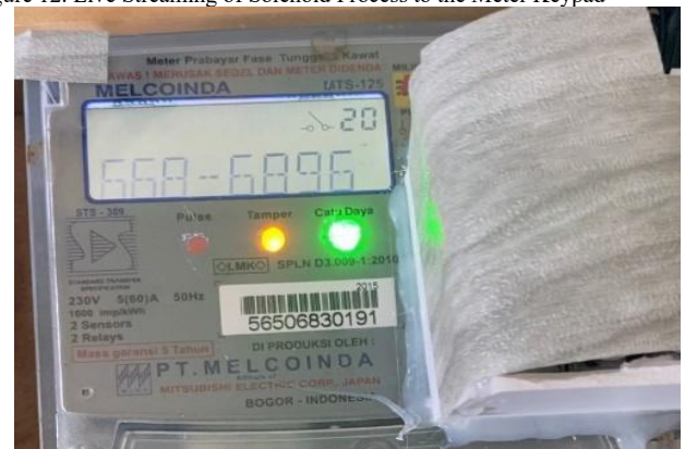
Figure 13. Solenoid Suppresses the Numbers Sent to the Database
