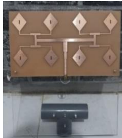
Figure 5. Fabrication results of diamond patch microstrip antenna i-slot array 4x2
