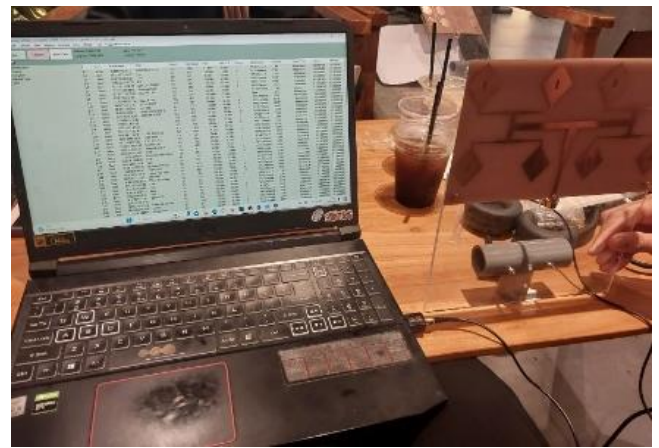
Figure 14. 4x2 array of diamond i-slot array patch microstrips for outdoor signal amplifier
