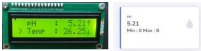
Figure 16. Integration Testing on pH Sensor
