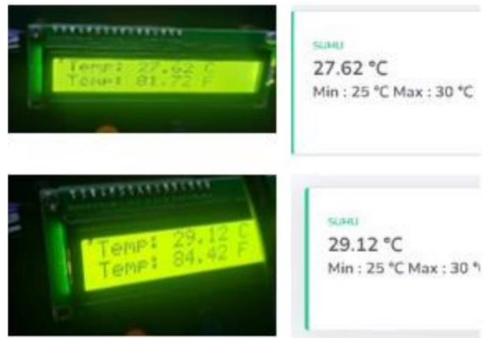
Figure 18. Integration Testing on DS18B20 Sensor
