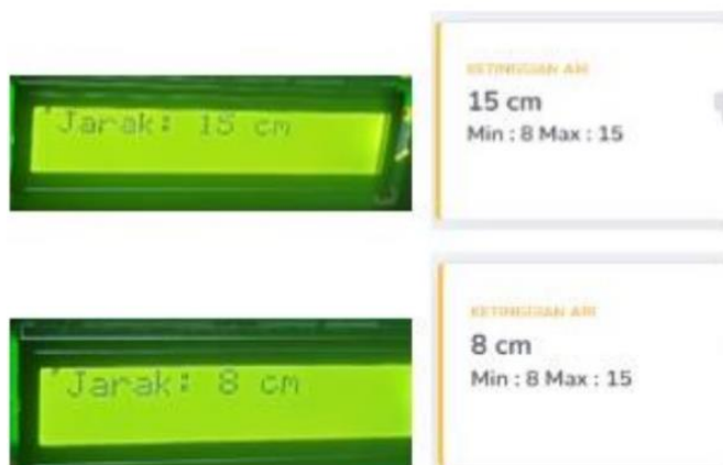
Figure 17. Integration Testing on Ultrasonic Sensor
