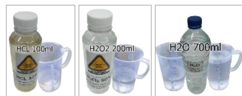
Figure 4. PCB etching solution mixture.
