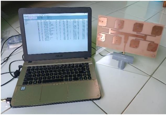
Figure 20. Truncated Corner Patch Without Disc Sector Slot 4x2 Array Microstrip Antenna for Signal Amplifier
