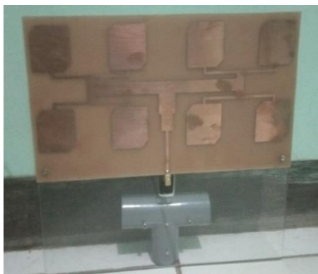
Figure 4. Fabrication Results of Truncated Corner Patch Microstrip Antenna Array 4x2
