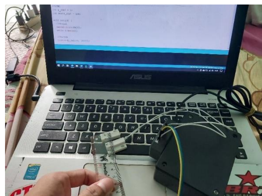
Figure 9. Testing of the magnetic switch sensor.
