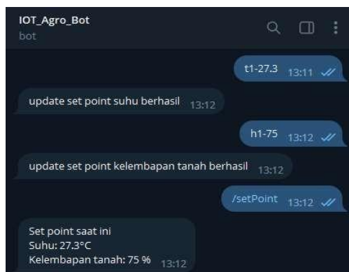
Figure 20. Temperature and humidity set point update command
