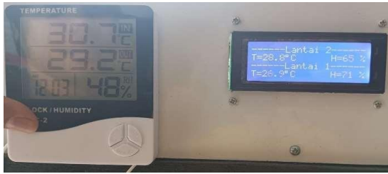
Figure 13. Comparison of DS18B20 temperature sensors on floor
