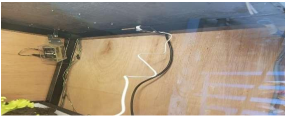
Figure 15. Location of the DS18B20 comparison sensor
