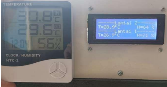
Figure 14. Comparison of 2 nd floor DS18B20 temperature sensors
