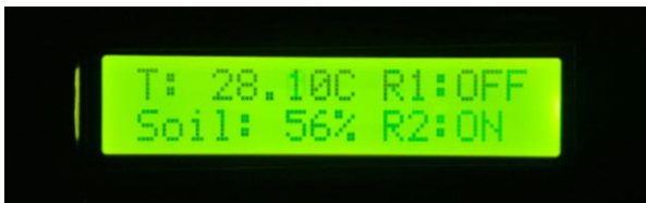
Figure 15. Sensor DHT11 Test (Relay Off)
