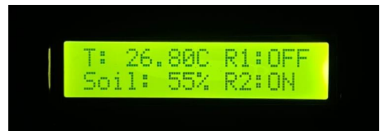
Figure 13. Soil Moisture Test (Relay On)
