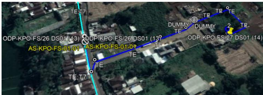
Figure 6. The fiber optic distribution route and ODP locations (ODP-KPO-FS/26 and ODP-KPO-FS/27) at the KPO-FS access segment
