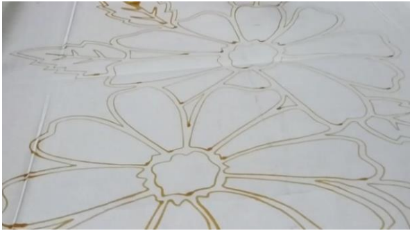
Figure 10. Batik Pattern Plotting Results with Temperatures Between 55-70°C
