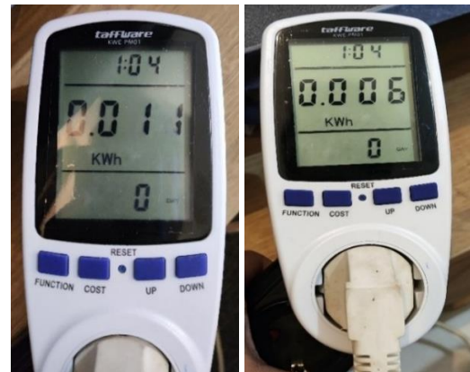
Figure 16 Test Results of wattmeter (a) without automatic lighting system (b) with automatic lighting system
