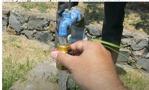
Gambar 15. Uji Fungsionalitas Sensor Water Flow
