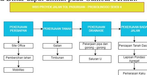
Gambar 2. Work Breakdown Structure
