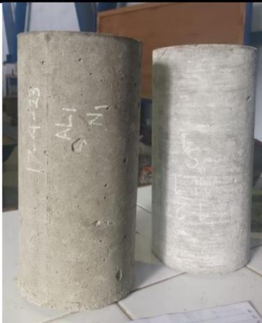
**Gambar 4.** (a) Curing air tawar, (b) Curing air laut
