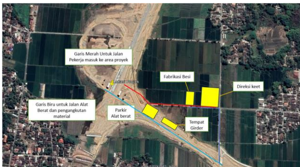
Gambar 10. Traffic Management proyek
