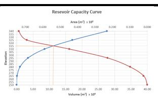
Figure 3.7 Reservoir Capacity Curve Source: Calculation Result, 2024
