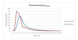
Figure 3.8 Flood Flood Routing Q1000th Source: Calculation Result, 2024
