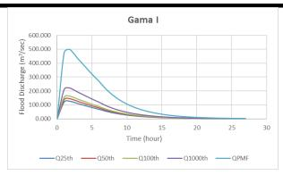
**Figure 3.6** The Gama I Curve Source: Calculation Result, 2024
