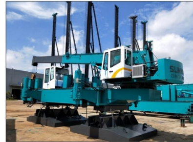
Gambar 4. Hydraulic Static Pile Driver
