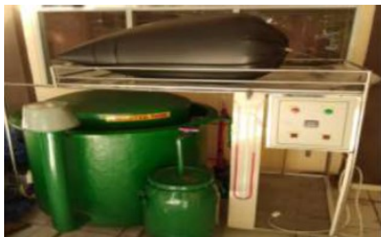
Figure 1. fixed dome Biogdigester [26]
