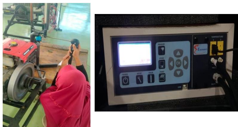
Figure 3. Emission testing using a gas analyzer
