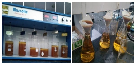
Figure 1. Coagulation and sedimentation of POME.
