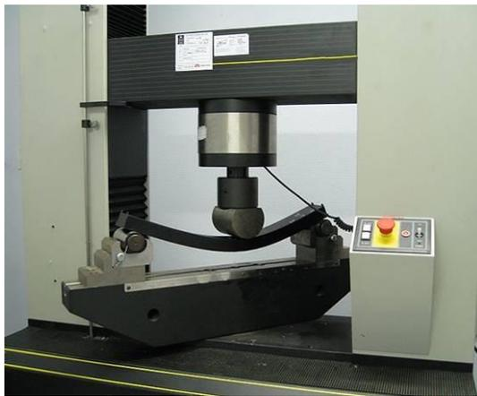
Gambar 2. Uji Bending [11]
