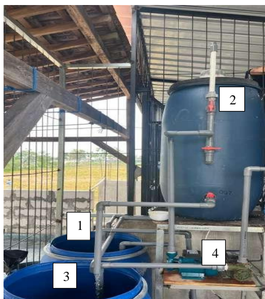
Gambar 2. Rangkaian alat filtrasi-adsorpsi
