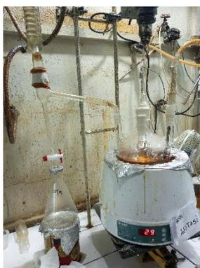
**Gambar 2.** Rangkaian alat distilasi larutan getah pinus
