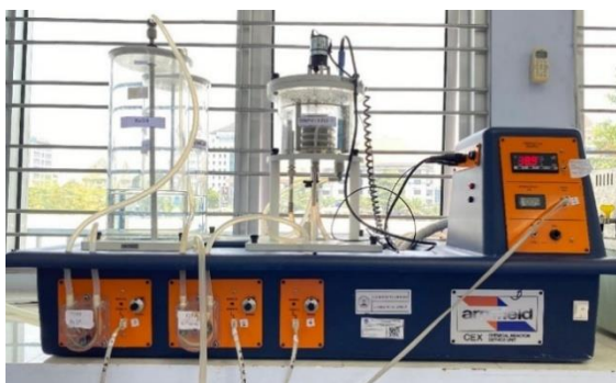
Gambar 1. Continuous Stirred Tank Reactor (CSTR) Armfield tipe CEM MkII
