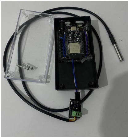
Gambar 1. Alat monitoring suhu Berbasis IoT
