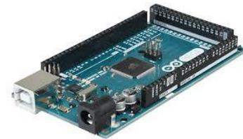
Gambar 3 Arduino Mega 2560
