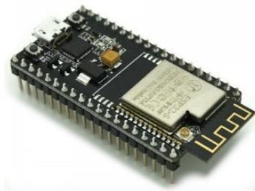
Gambar 3. Modul ESP32
