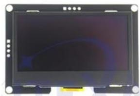
Gambar 7: OLED 2.42" I2C Display
