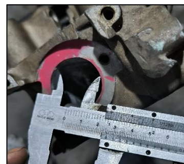
Gambar 3. Intake Port 26,5 mm
