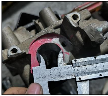
Gambar 4. Intake Port 28,5 mm
