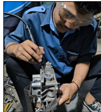
Gambar 1. Proses Porting Head Intake dan Exhause
