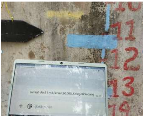
Figure 5. Comparison of Results from the WhatsApp Bot with Measurements from the 11 m 3 Tank
