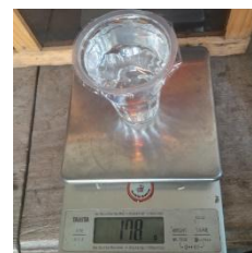
Figure 4. Water Volume Accuracy Test Documentation
