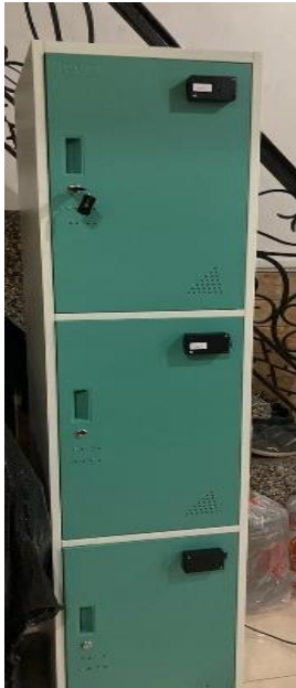
Figure 6. Front view of the smart locker hardware implementation
