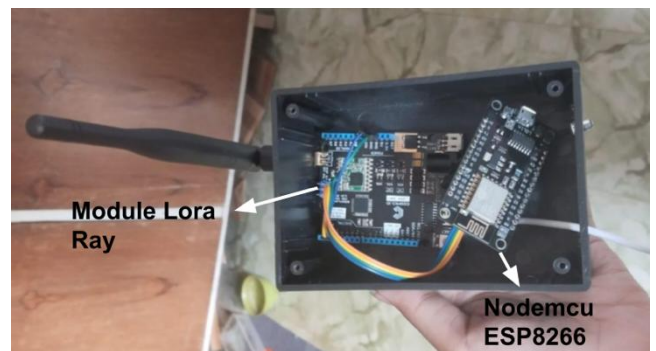
Figure 5. Server Node Circuitry
