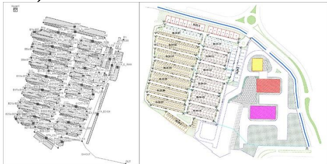
Gambar 6 Permodelan SWMM Cluster Alstonia (Sumber : Perhitungan, 2025)
