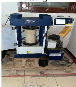
Image 3.17. Concrete Compressive Strength Testing
